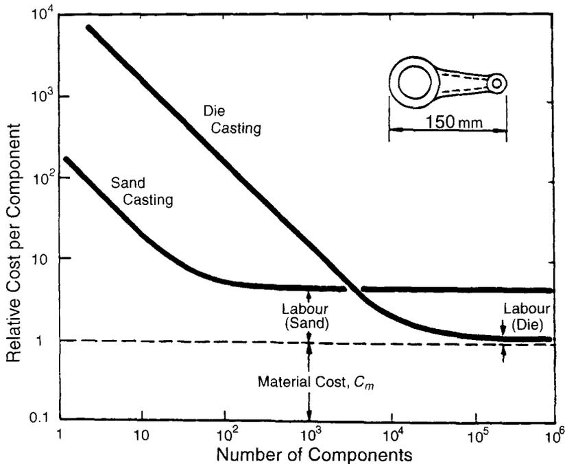
**Fig. 11.38** The best choice of casting (or machining or forging) process depends on batch size. Sand casting requires cheap equipment but is labour intensive. Die casting requires more expensive equipment, but is faster. The data shown here are for an automobile connecting rod.
