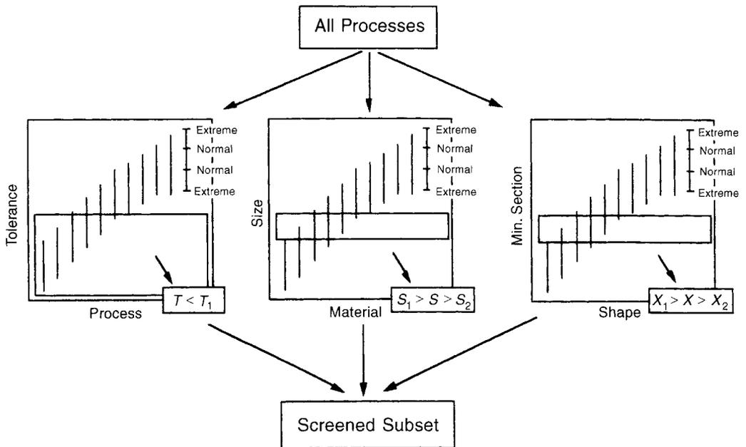
**Fig. 11.35** Computer-based screening. The attributes of processes are plotted as bar-charts, isolating processes which can handle a given material class, create a given class of shapes, and meets the design requirements on size, tolerance and minimum section.
