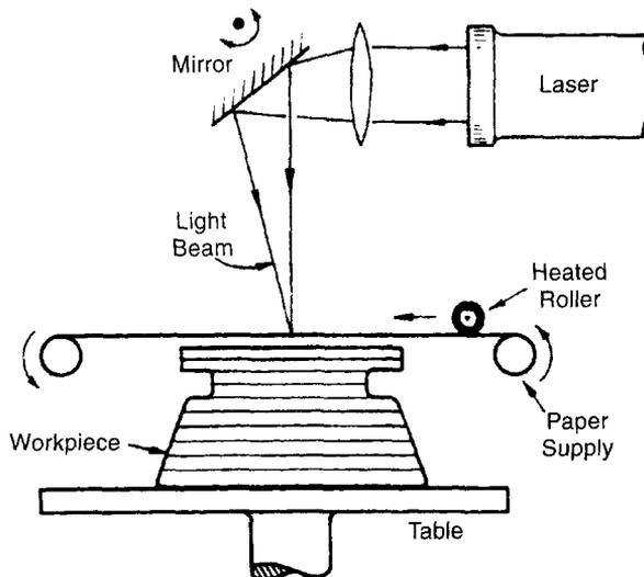
**Fig. 11.25** Laminated object manufacture (LOM), a rapid prototyping method by which a solid body is created from layers of paper, cut by a scanning laser beam and bonded with a heat-sensitive polymer.
