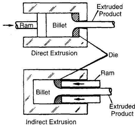
**Fig. 11.11** Extrusion. Material is forced to flow through a die aperture to give a continuous prismatic shape. Hot extrusion is carried out at temperatures up to  $0.9T_m$ ; cold extrusion is at room temperature.
