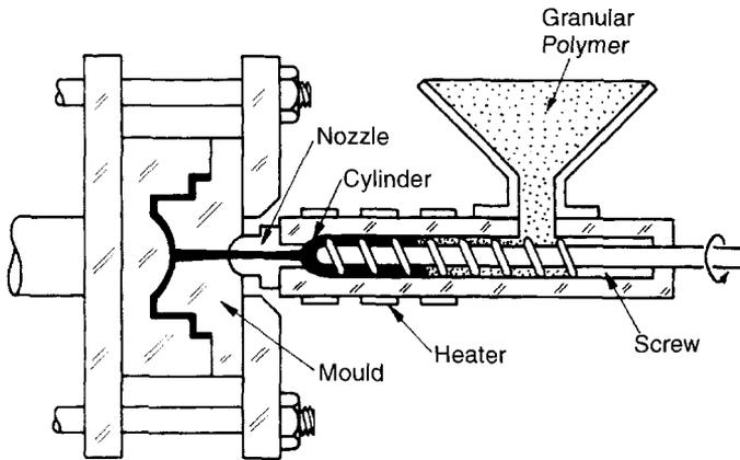
**Fig. 11.7** Injection-moulding. A granular polymer (or filled polymer) is heated, compressed and sheared by a screw feeder, forcing it into the mould cavity.
