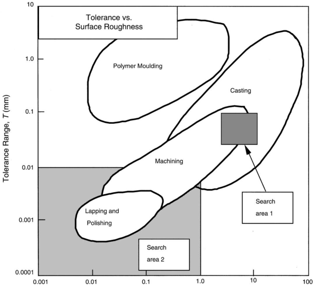
**Fig. 11.28** A schematic illustrating the idea of a process-selection chart. The charts have process attributes as axes; a given process occupies a characteristic field. A design demands a certain set of processes attributes, isolating a box ('Search Area 1') or a sub-field ('Search Area 2') of the chart. Processes which overlap the search areas become candidates for selection.
