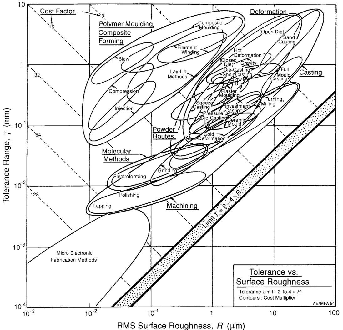
**Fig. 11.33** The tolerance–roughness chart.
