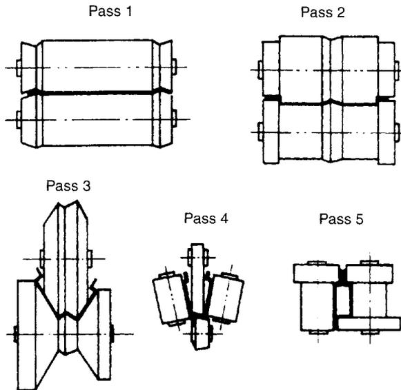
**Fig. 11.9** Rolling. A billet or bar is reduced in section by compressive deformation between the rolls. The process can be hot ( $T > 0.55T_m$ ), warm ( $0.35T_m < T < 0.55T_m$ ) or cold ( $T < 0.35T_m$ ).
